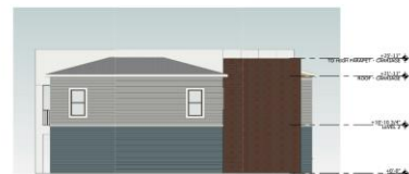
2 NORTH ELEVATION - CARRIAGE BLDG SCALE: 1/8" = 1'-0"
