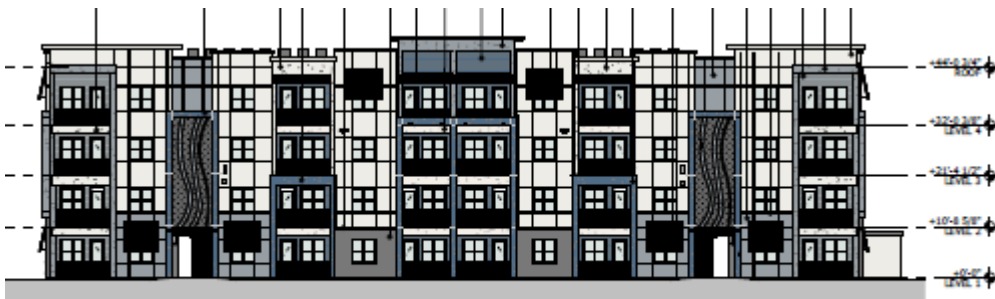
BLDG TYPE II - LEFT ELEVATION SCALE: 1/8" = 1'-0"
