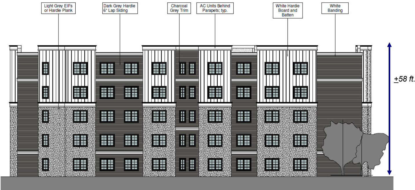
1 North Elevations Bld 2 - Flat Roof Option 3/16" = 1'-0"
