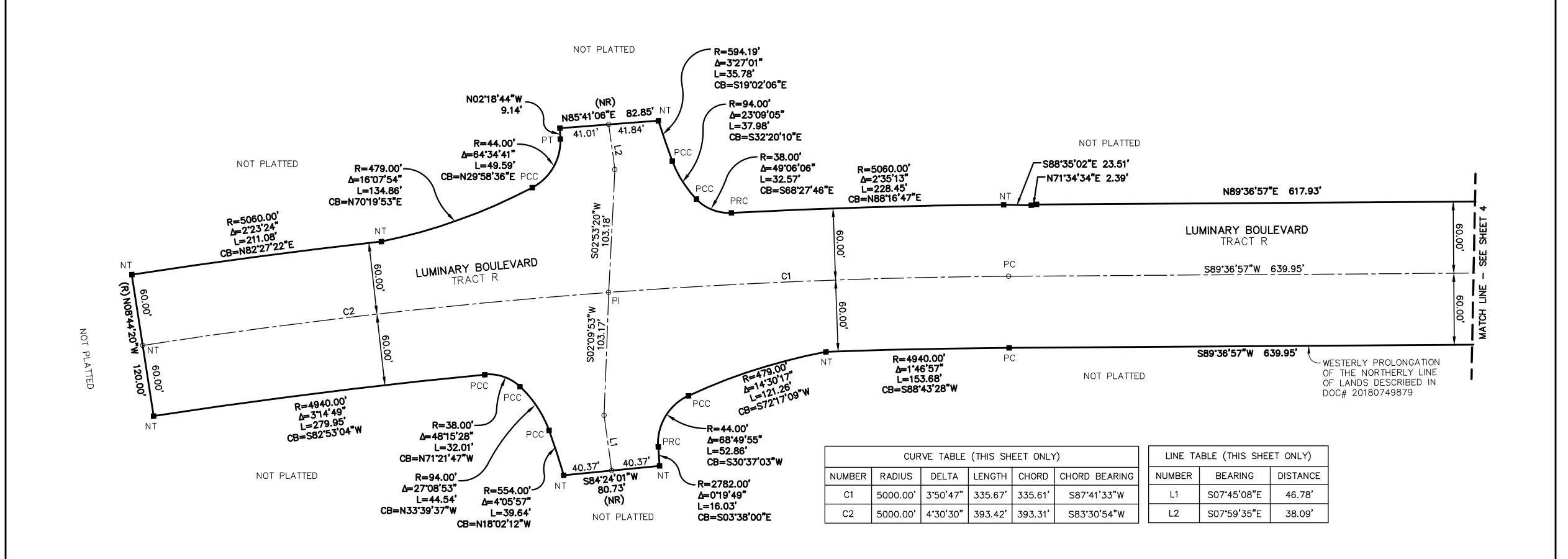
The features and linework shown hereon are in grid relative to National Geodetic Survey control point "Lance" (PID AJ2445), Northing 1477081.39, Easting 575759.46 Florida State Plane Coordinate System, Florida East zone, 1983 North American Datum, 2011 adjustment average combined scale factor: 0.99994883912 (1.00005116349757). All dimensions are Grid dimensions in U.S. Survey Feet, based on said Florida State Plane Coordinate System, Florida East zone, 1983 North American Datum, 2011 adjustment.
